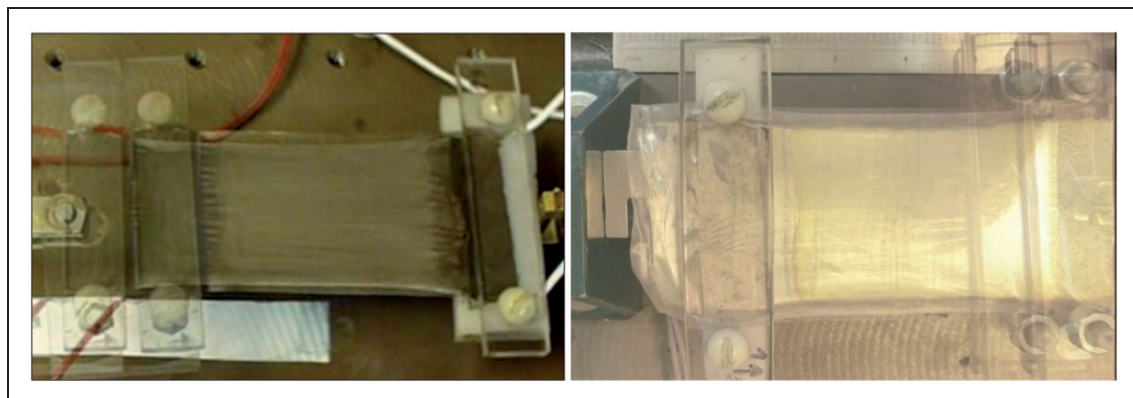
Figure 5. Superimposed images of unstretched ( \lambda = 1 ) and stretched ( \lambda = 1.27 ) DE film (left: graphene, right: PolyPower) demonstrates the lateral contraction of the film. greater contraction can be observed for graphene than for PolyPower.
